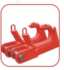
**3- Hook Fast Disentangled:** It secures rope connection between buoy and ship. The hook that is manufactured to hold ship's ropes safely ensures the rope is freed which is broken away by the moving part over the load shaft. Hooks that are made of ST52-3 materials are certified by the Turkish Lloyd project and test. There are products between the range of SWL 50 ton – SWL 200 ton.
