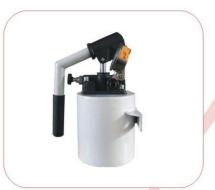
**2-Hydraulic Manual Operator**: It secures conveying the oil to the hydraulic valves and opening and closing them. By 0-40 bar pressure adjustment it secures opening and closinf valves safely. It produces maximum 0-100 bar pressure. It has 1lt-3-lt capacity.
