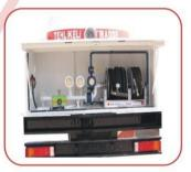
**8-Mobile Hydraulic Operator Adapter:** Adapter is mounted on LPG tanker. It supplies not being of any hydraulic operator on the tanker. In general, by the adapter used in tankers among installations intervention in hydraulic valves of tanker is only made in facility. Adapter is made of brass casting and steel materials. It operates without leakage thanks to sealing elements.
